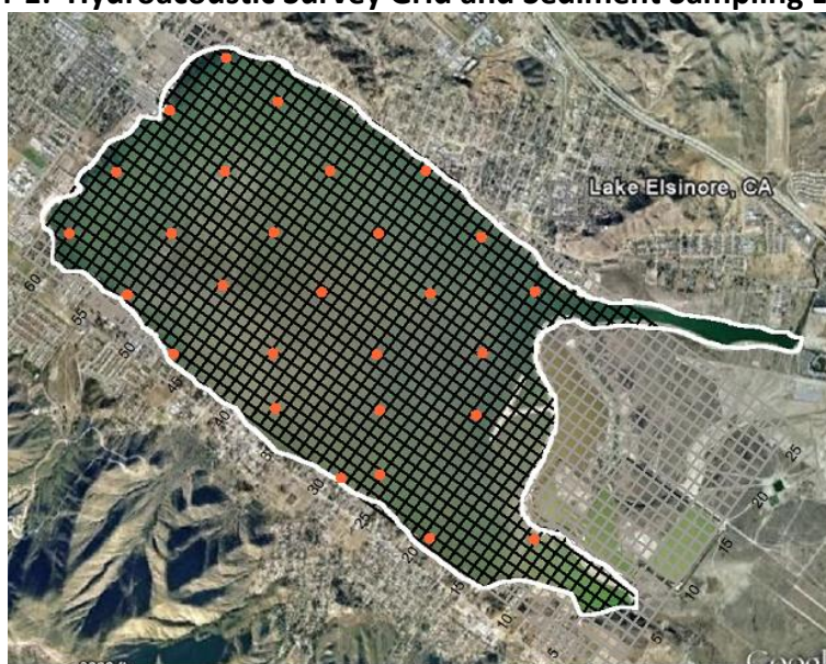
Figure 4-1: Hydroacoustic Survey Grid and Sediment Sampling Locations
