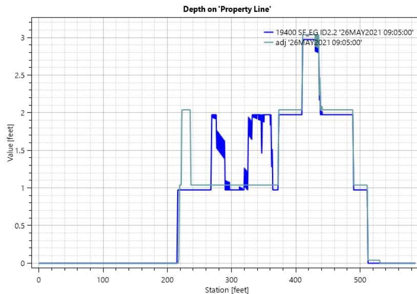
Figure 3b – Flow Depth at Section A: Property Line
