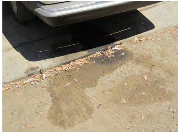
Photograph 14. Oil staining on soil and concrete pad at 29445 3 rd Street.
